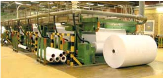
*Sheet cutter and butt rolls*
