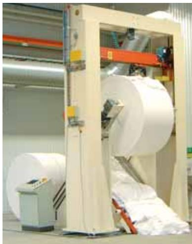
*Roll cutter with tilting table for narrow reels*
