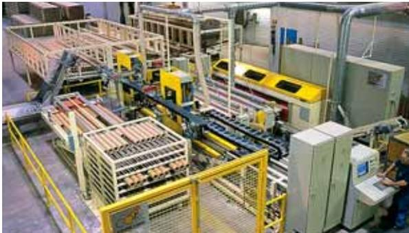
*Automatic core cutter with metal end capping and set cart loading*
