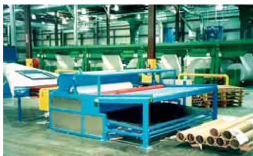
Core stripper connected to a trim system
