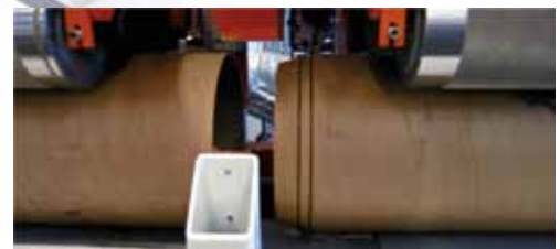
Core Joining Station – Adhesive Applied on Male Cone
