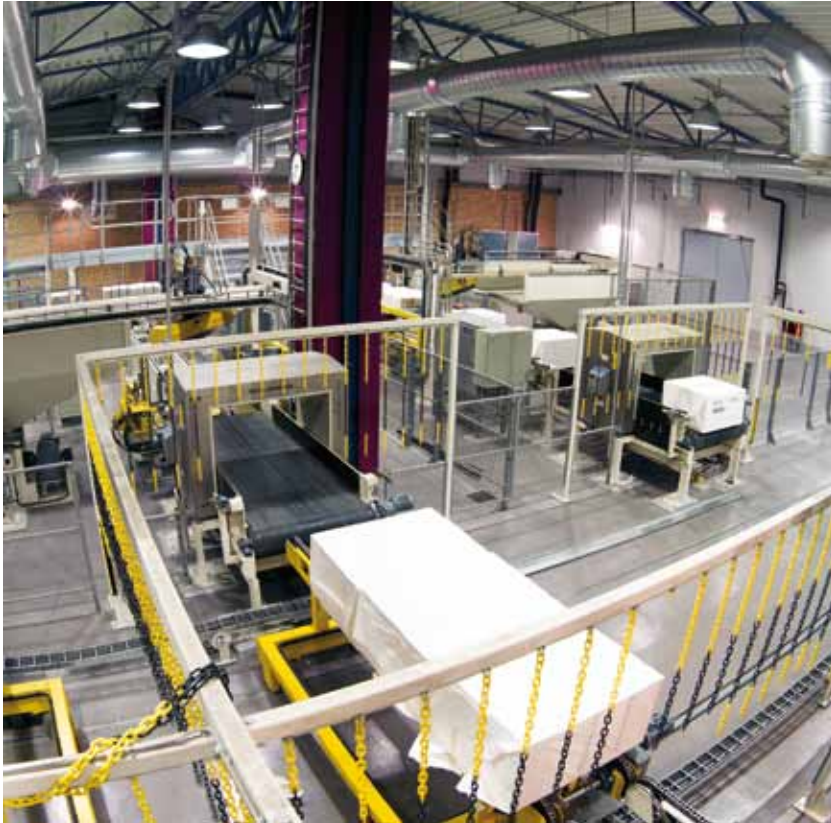
Automatic Pulp Bale Handling – Including Unit De-wiring, De-stacking and Single Bale de-wiring
